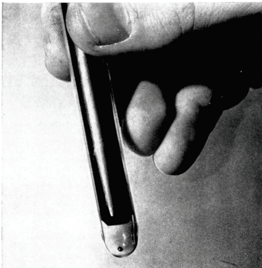
PELLET IN VACUUM TUBE, along with ferrite magnetic core, is inserted in apparatus shown on preceding page. There the tube is surrounded by liquid helium to increase vacuum.
